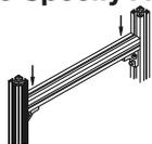
Allowable load per one bracket is calculated with one beam extrusion between two vertical extrusions supported by a bracket under each side of the beam as shown on the left-side figure.
