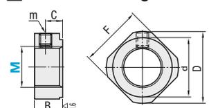
⚠ Tighten the set screw after inserting the Thread Protector.
