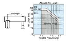
For clamping, allow 3 mm or more before the stroke end.
