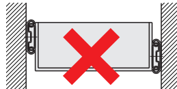
Slide rails are not horizontally aligned.
